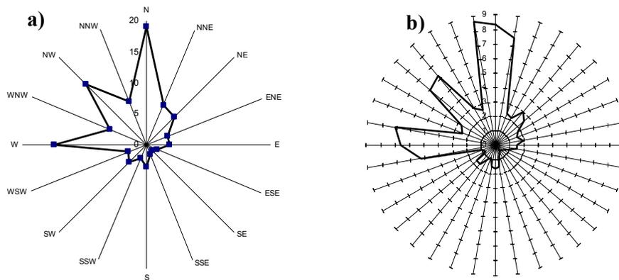
Figure 2. Wind roses for station Pernik (1991-2000) built from the processed data.
