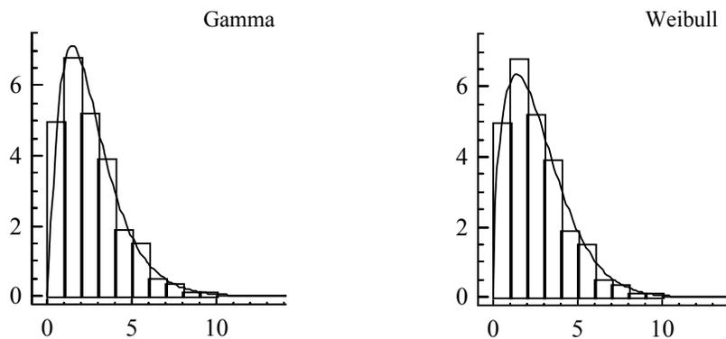
Figure 4. Fitting the processed data wind speed histogram of station Pernik (1991-2000).
