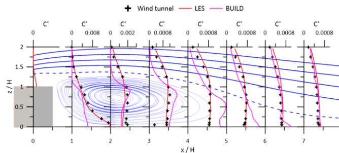
**Figure 7.** Evolution of the concentration field dimensionless from the experiment (black cross), the LES simulation (red line) and the BUILD simulation (pink line). In the background, streamlines from the LES simulation.
