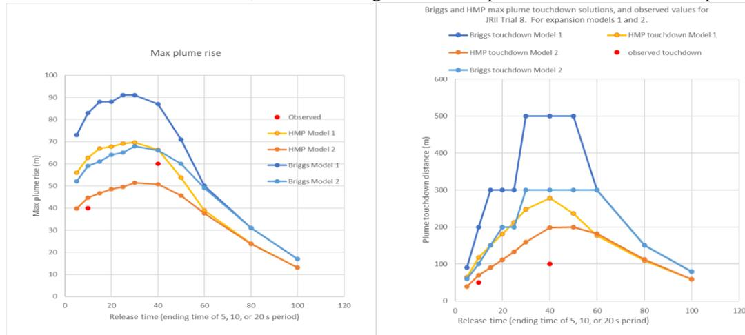
**Figure 2.** Observed and modeled maximum plume rise (left) and touchdown distance (right), calculated using emissions rates for 11 time segments after release was initiated. Red dots are observed.
