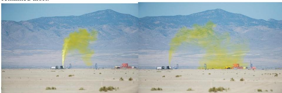
**Figure 1.** Jack Rabbit II Trial 8 plume 12 s (left) and 28 s (right) after chlorine release begins. The plume center at maximum rise is about 40 m.
