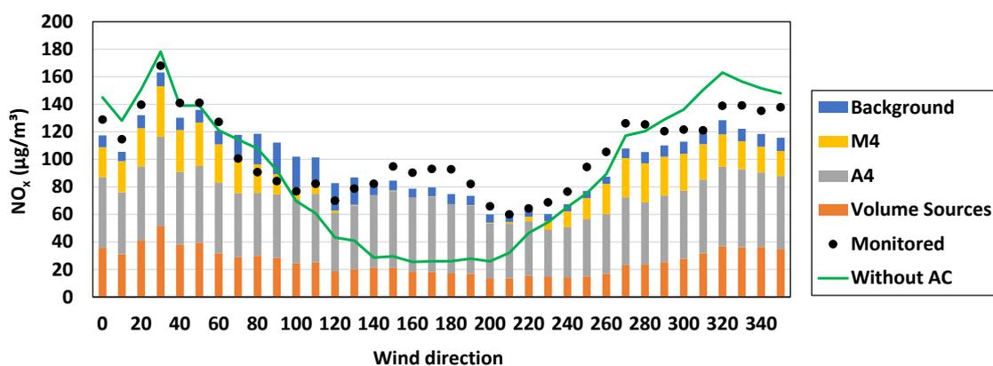
**Figure 4.** NO<sub>x</sub> source apportionment by wind direction using the new approach at the HS5 site.
