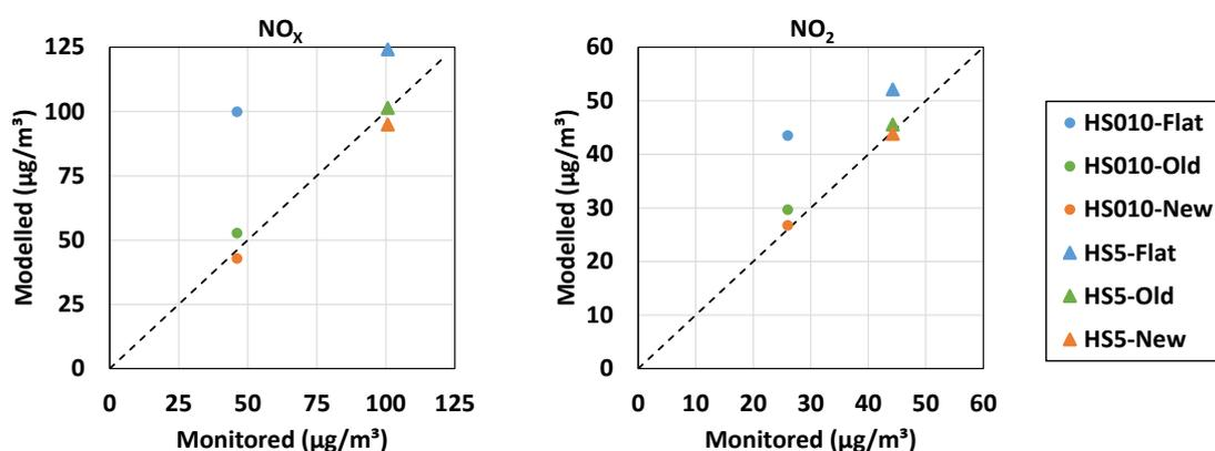
**Figure 3.** Modelled vs monitored annual average NO<sub>x</sub> and NO<sub>2</sub> scatter plots at the HS010 (circles) and HS5 (triangles) sites for the ‘Flat’ (blue), ‘Old’ (green) and ‘New’ (orange) modelling approaches.
