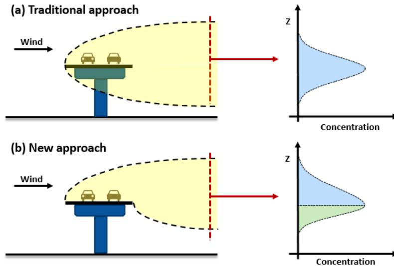
**Figure 1.** Schematic of the traditional (a) and new (b) approach to modelling an elevated road source in ADMS.
