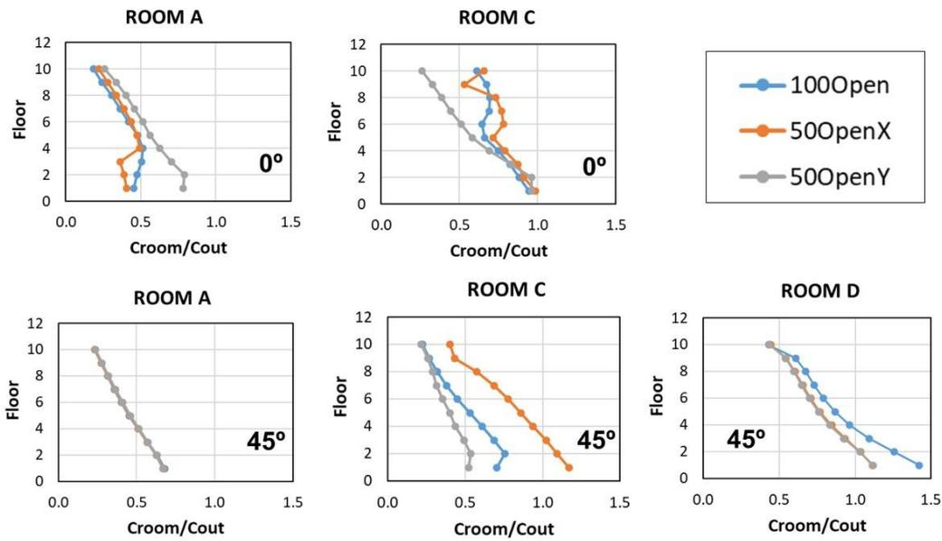
**Figure 2.** Ratio between the average concentration at different rooms (Croom) and the spatially-averaged concentration at pedestrian level in the street (Cout) for both wind directions and different arrangements of open/closed windows.
