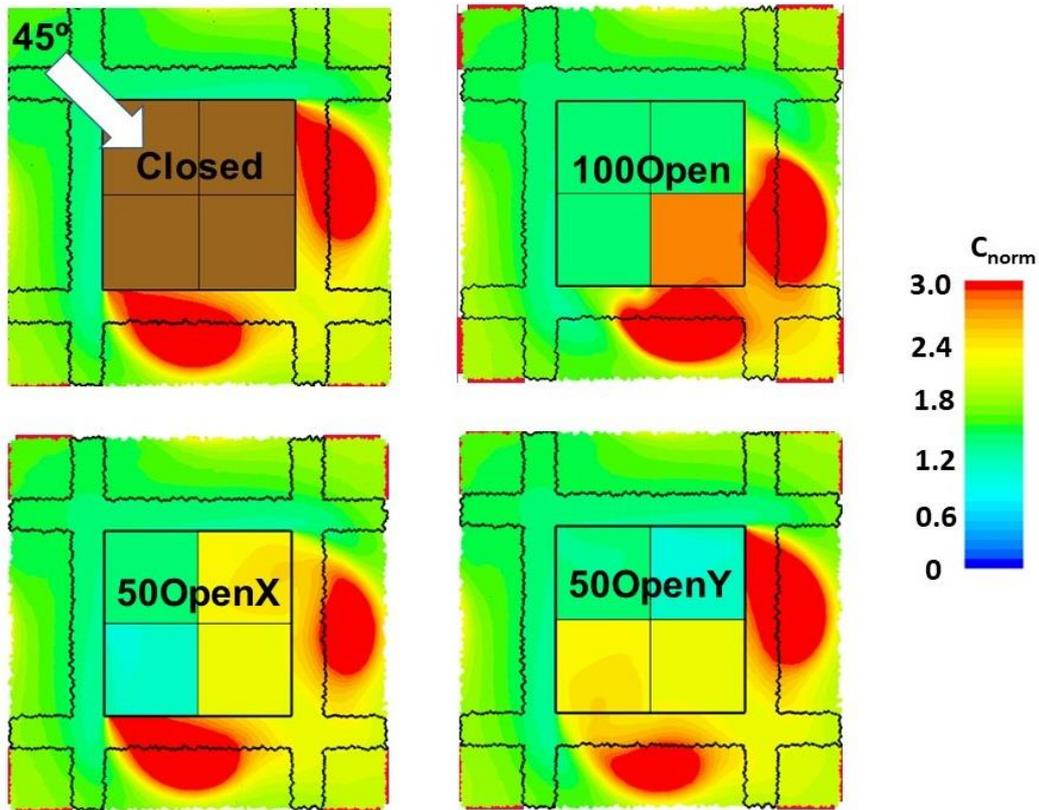
**Figure 4.** Normalized concentration around and inside the target building at 3m height for different configurations of open/closed windows and for a wind direction of 45°. Arrow indicates wind direction above roof level.
