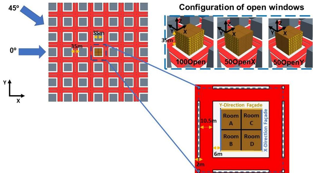
**Figure 1.** Configuration of buildings studied and details about the target building with windows. Open windows are coloured in yellow and traffic emissions are coloured in red.
