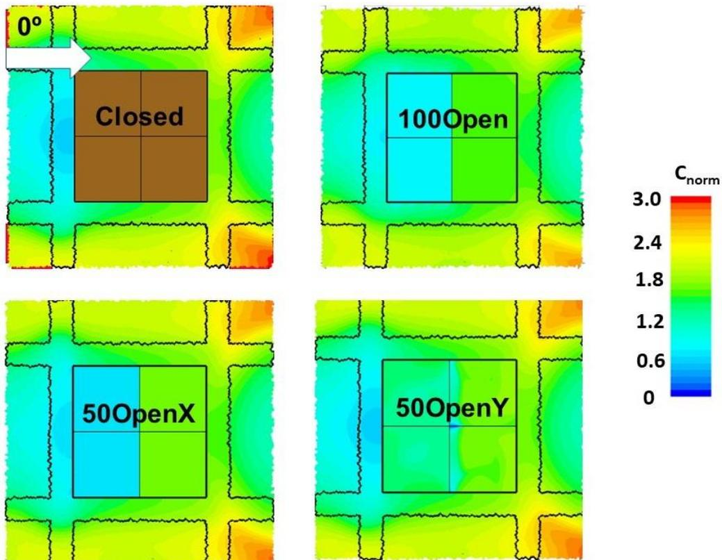
**Figure 3.** Normalized concentration  $C_{norm}$  around and inside the target building at 3m height for different configurations of open/closed windows and for a wind direction of  $0^\circ$ . Arrow indicates wind direction above roof level.
