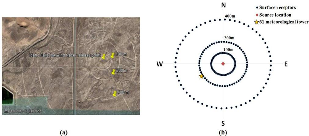
**Figure 1.** (a) Idaho Falls experiment site view (b) Schematic of Idaho Fall field with the location of the source and measuring sensors
