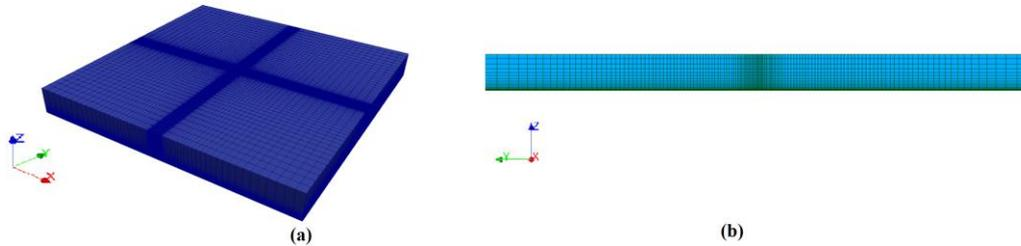
**Figure 2.** Mesh representation ( $L=W=900$  m,  $H=60$  m) for run-10 of Idaho Falls experiment (a) 3-dimensional view (400000 cells) (b) Vertical mesh. Close to the release point, the cells measure  $0.72$  m  $\times$   $0.72$  m  $\times$   $1.2$  m. The mesh is refined near the ground and the vertical resolution varies from  $0.5$  m to  $7$  m.
