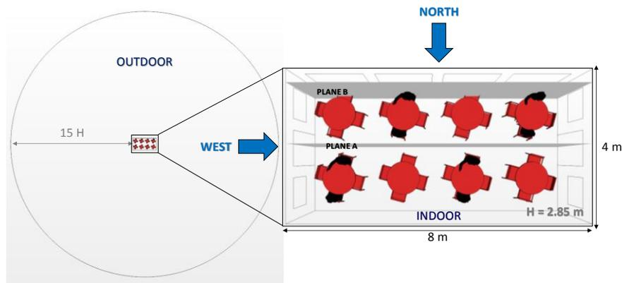
**Figure 1.** Geometric model: global and local dimensions (Ordenanza, 2013) and layout of the people inside the terrace.
