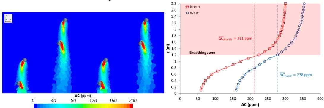
**Figure 4.** Left)  $\Delta\text{CO}_2$  high resolution map at 1.2 m height (onset of breathing zone). Right)  $\Delta\text{CO}_2$  surface average profiles during the steady state for both wind directions.
