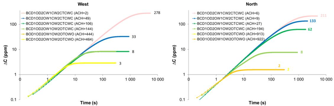
**Figure 3.** Time evolution of volume average  $\Delta\text{CO}_2$  concentration for different values of ACH for: left) West wind direction and right) North wind direction.
