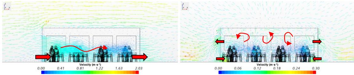
**Figure 5.** Tangential component of the velocity field on plane A in BCD1OD2OW1CW2CTCWC scenario for: left) West wind direction and right) North wind direction.
