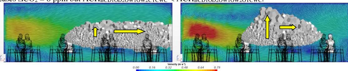
**Figure 6.** Line integral convolution of tangential component of velocity field on plane B and recreation of exhaled  $CO_2$  by one of the people (cells in gray color) for West wind direction in: left) BCD1OD2OW1OW2CTCWC scenario and right) BCD1OD2OW1OW2OTCWC scenario.
