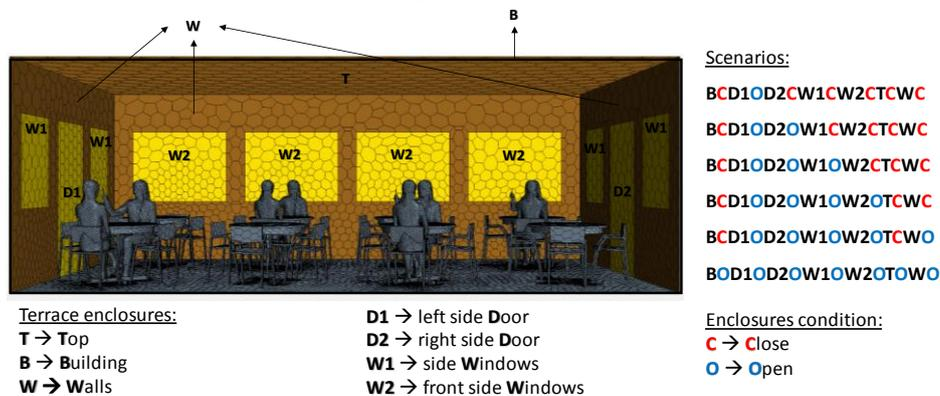
**Figure 2.** Meshing on indoor surfaces and set of virtual scenarios.
