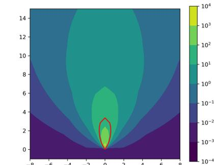
Example of inhalation dose map (mSv) obtained by simulation. The red isoline correspond to the threshold exceedance of 50 mSv.
