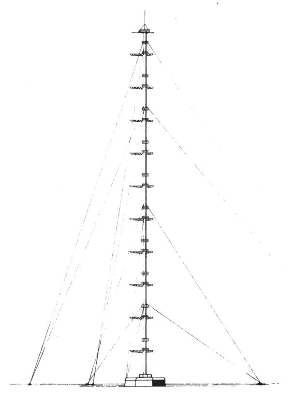
Figure 1 General contruction of the 213 m meteorological mast at Cabauw in The Netherlands
